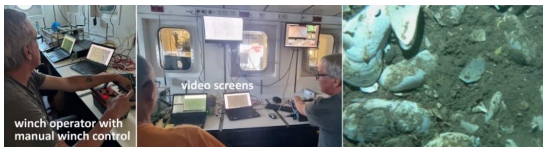
Fig. A5.2 (from left to right) Winch operator in the TV-GBC control laboratory. The video helps to select sampling sites. Screenshot showing a sampling site shortly before the box corer was placed on the seabed.
