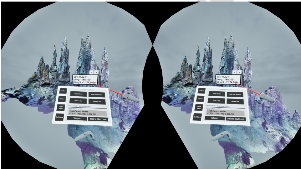
(b) A screenshot of the HMD VR setting showing what is being rendered for both eyes. The image also shows the menu widget attached to the left HTC Vive controller and the “pointer ray” emanating from the right controller.
