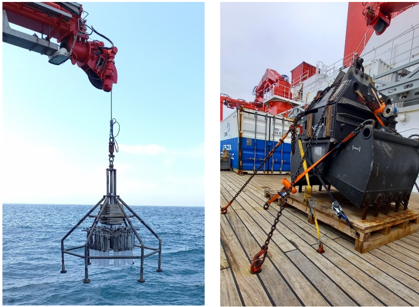
Fig. 5.15 a) Charged multicorer on its way down to the seabed using the small sliding beam (left). b) TV-grab fixed on pallet after revision by SONNE's scientific technical service (right). Photos: C. Lüter.
