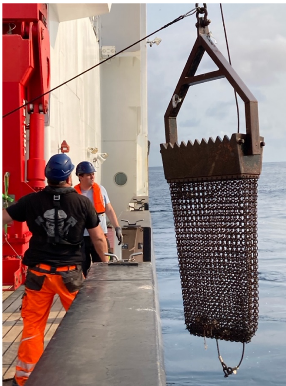
Fig. 5.6 Deployment of a GEOMAR chain bag dredge during SO307. Photo: J.G.
