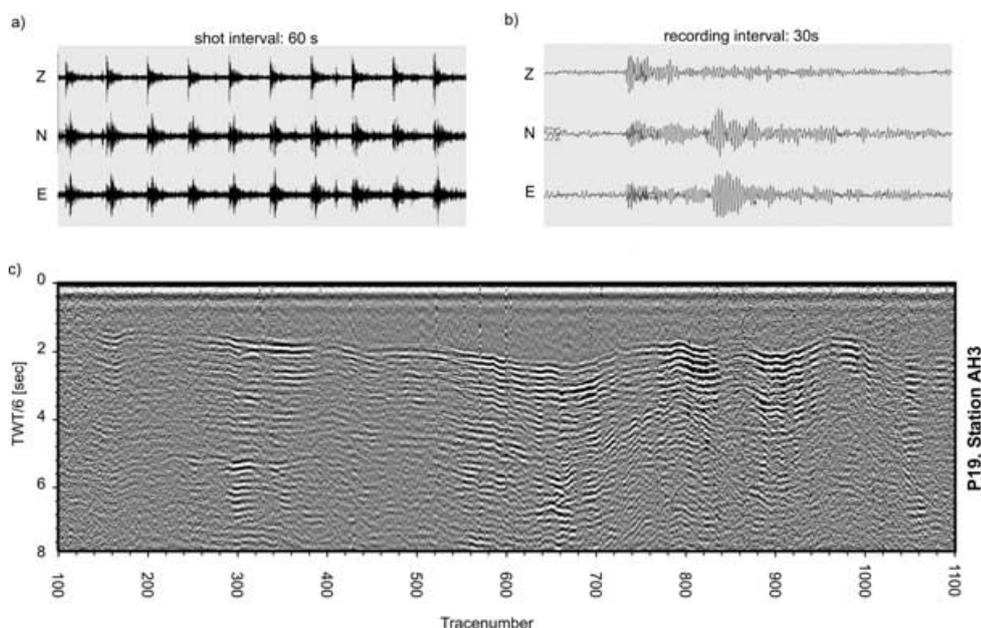
**Figure 2.** (a) Z, N and E components of airgun signals having a shot interval of 60 s recorded onshore. (b) Zoomed-in seismogram of one single airgun shot. The shown recording interval is 30 s. (c) Example of a seismic section of an onshore station (AH3) located southwest of Merapi volcano in Central Java. It shows the good data quality of the airgun profile P19 recorded onshore. The first onset of each trace of the coast-parallel profile can be picked at this onshore station.
