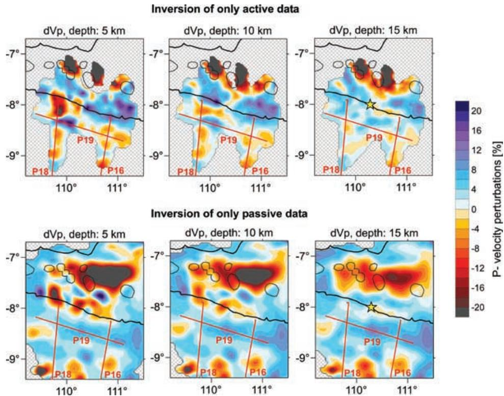
**Figure 3.**  $P$ -velocity anomalies after inversion of only active and only passive seismic data presented in horizontal sections at 5, 10 and 15 km depth. The black lines are the coastline and volcanoes located in Central Java. The airgun profiles are plotted with red lines.
