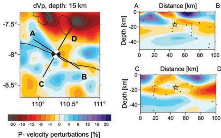
**Figure 7.** The left diagram shows a zoomed-in horizontal section of the joint inversion at 10 km depth. The two black lines indicate the positions of vertical sections crossing the BGR hypocentre of the Java earthquake in 2006 May. Black dots mark earthquake hypocentres of the MERAMEX catalogue.
