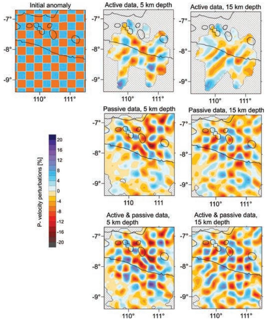
**Figure 6.** Comparison of the checkerboard tests for active, passive and combined data sets. The upper left image is the initial shape of anomalies with amplitudes of  $\pm 7$  per cent. Noise of 0.15 s rms was added to the data in all cases. The 1st, 2nd and 3rd rows show results of reconstruction for the active, passive and combined data sets. Here, we present the results at two depths: 5 and 15 km.
