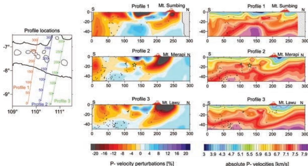
**Figure 5.** Result of the joint inversion for the  $P$ -velocity model presented in vertical sections. Profile locations are shown in the map on the left. The middle column presents relative perturbations of  $P$ -velocity; plots on the right show absolute velocities. Black dots mark hypocentres of the MERAMEX catalogue, the star in profile 2 marks the hypocentre of the Java earthquake in 2006 May.
