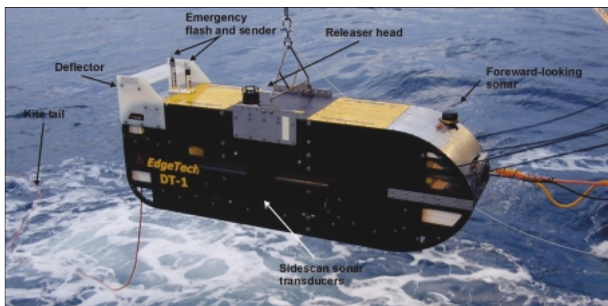
Figure 1: The DTS-1 side-scan sonar towfish during deployment.
