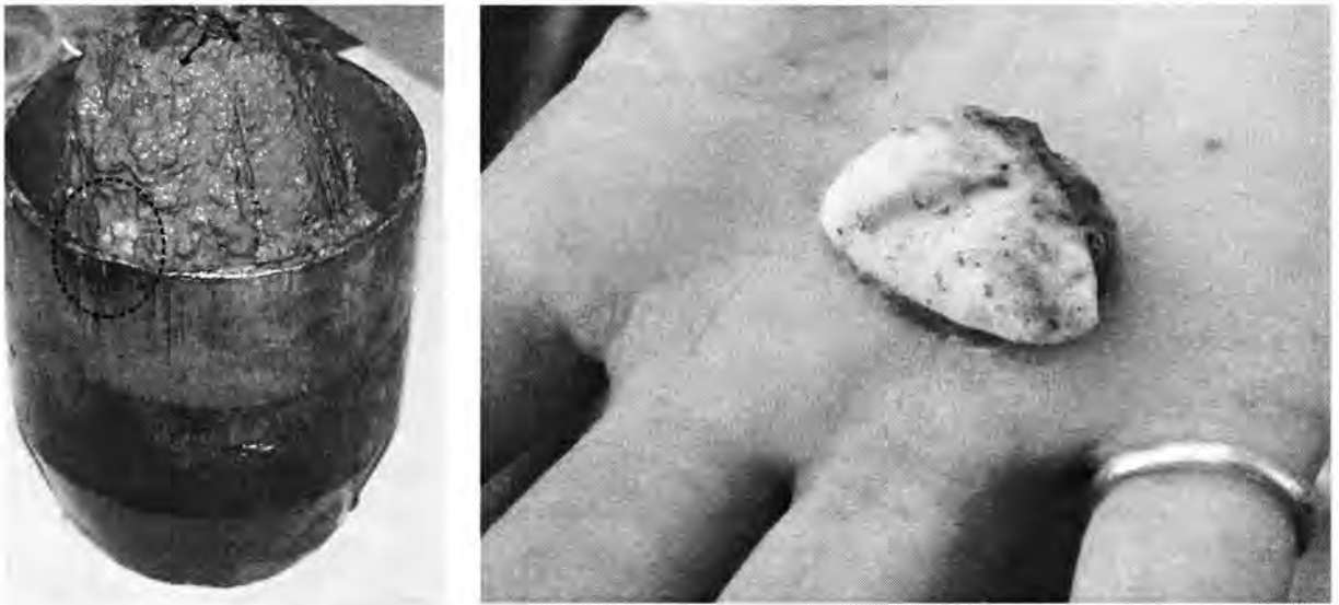
Figure 4.1.13: Small chips of gas hydrates in a gravity corer form Batumi Seep.
