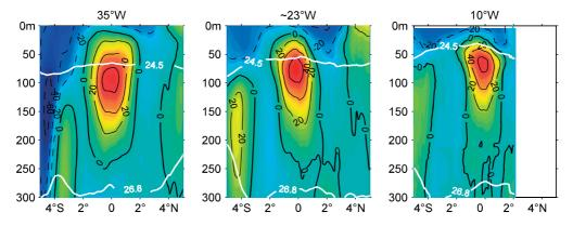
**Figure 2.** Mean zonal velocity [color shading and black contours (cm/s)] and potential density surfaces 24.5 and 26.8 (white solid lines) along three meridional sections: 35 °W, ~23 °W, and 10 °W (after Brandt *et al.*, 2006; Hormann and Brandt, 2007; Kolodziejczyk *et al.* 2009).
