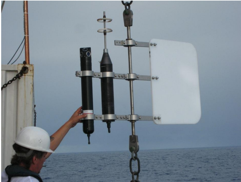
Figure 8.4: Picture of the vane system for mooring M1 with one Aquadopp HR profiler and one MAVS.
