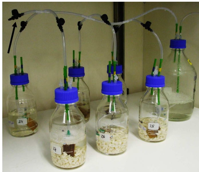
Figure 2.3 Set-up for sub-experiment two showing the 2400 ppm \text{CO}_2 treatment as well as its blanks without corals (blanks in the back). Valves (black) directed to each bottle allowed adjusting of the bubbling. One valve served as pressure relief valve (arrowed). Using the two litres bottle as gas wash bottle (in the back) the air was moisturized before running to the treatment bottles.
