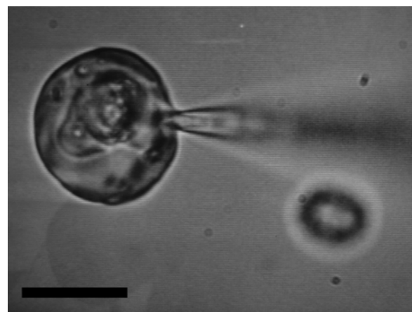
Fig. 33 Exemplary picture of a patch pipette sealed to a protoplast of C. pelagicus . Scale bar 10 \mu m
