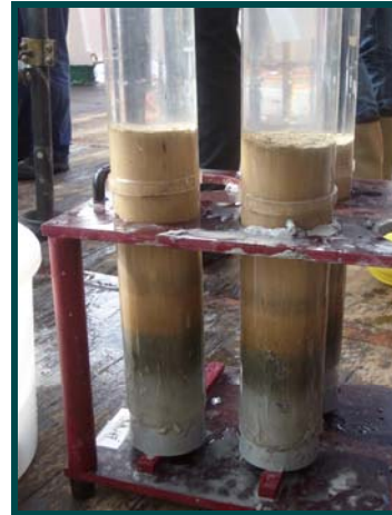
Figure 2b: Sediment samples from the Eastern Mediterranean deep-sea sediment, recovered by a multiple corer.
