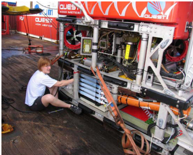
Fig. 2.1, The KIPS system mounted on the tool sled of the ROV QUEST (MARUM/Univ. Bremen) during cruise MARSÜD (M64/1). From Haase et al. (2005).
