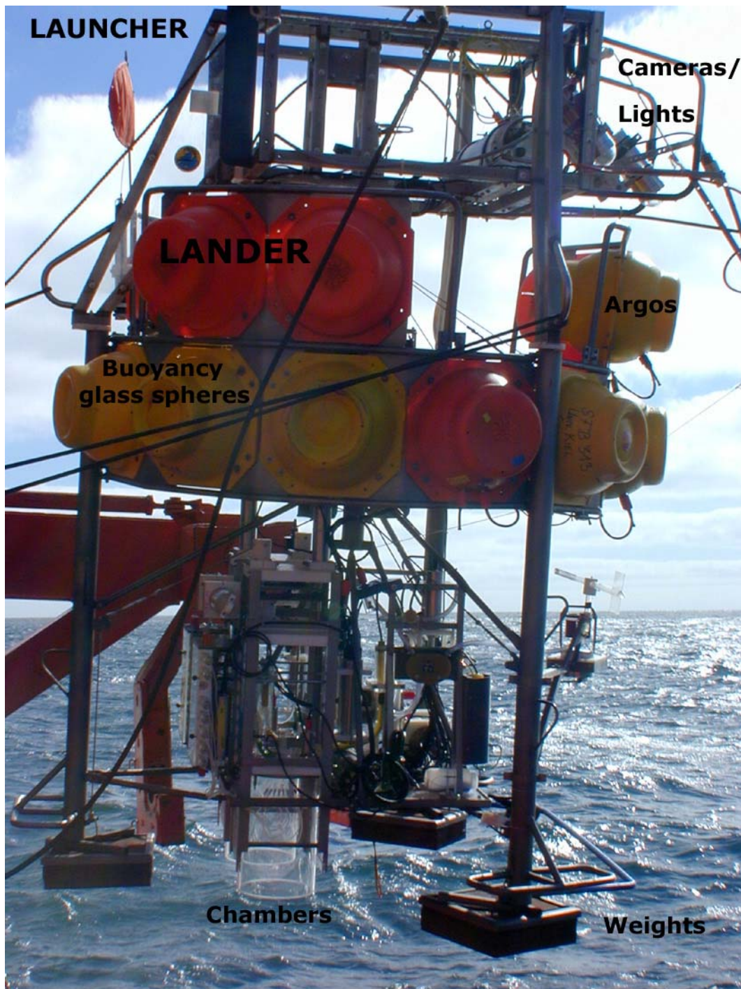
Fig.5.4.1: FLUFO attached to the launcher during deployment.
