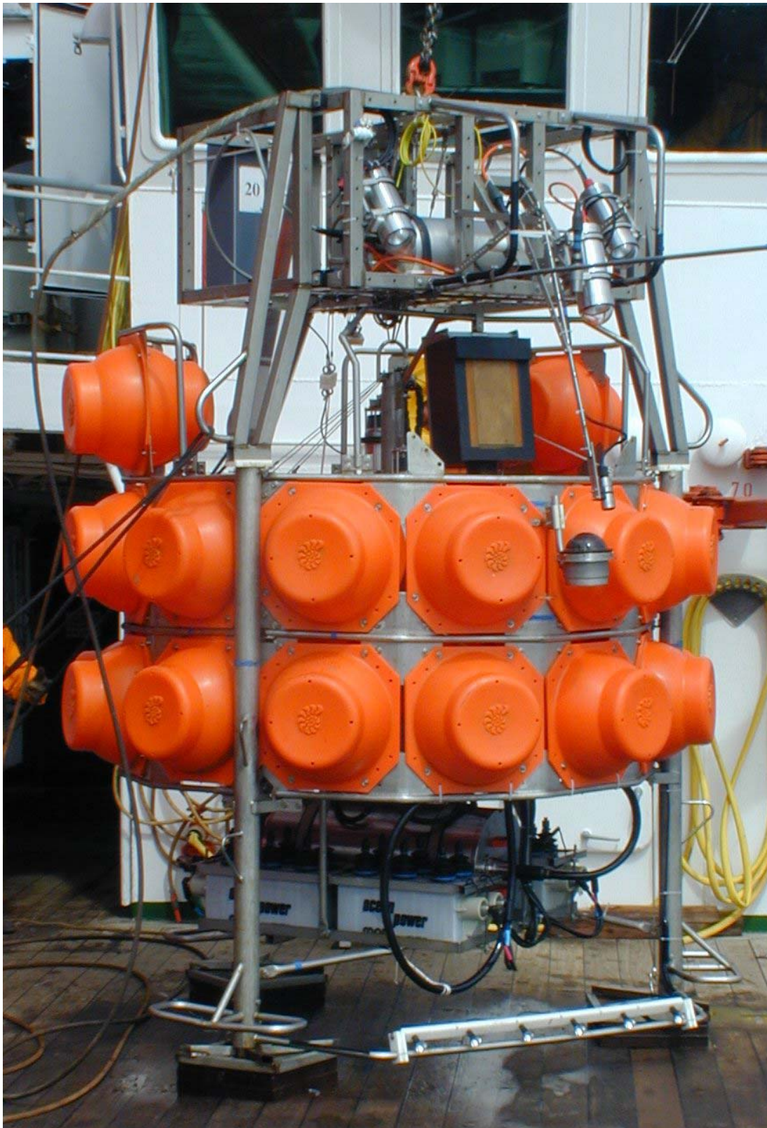
Fig. 5.3.5.2: View of the GasQuant Lander with launcher on top ready for deployment. The tool frame at the base of the lander carries four deep sea batteries and the SEE electronics in a titanium barrel. A compass, observed by one of the two launcher-cameras, was used to control the lander heading during the deployment.
