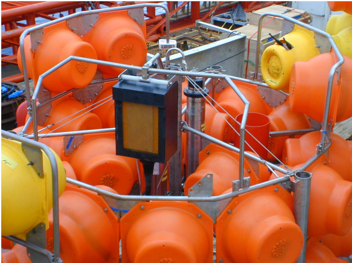
Fig. 5.3.5.3: The pressure resistant 180 kHz transducer of the GasQuant system fixed in a cardanic frame.
