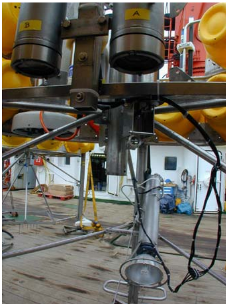
Fig. 5.5.4: View from below on the 12 bottles of the cone-shaped trap after recovery.
