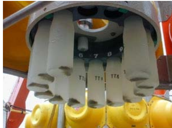
Fig. 5.5.4: View from below on the 12 bottles of the cone-shaped trap after recovery.
