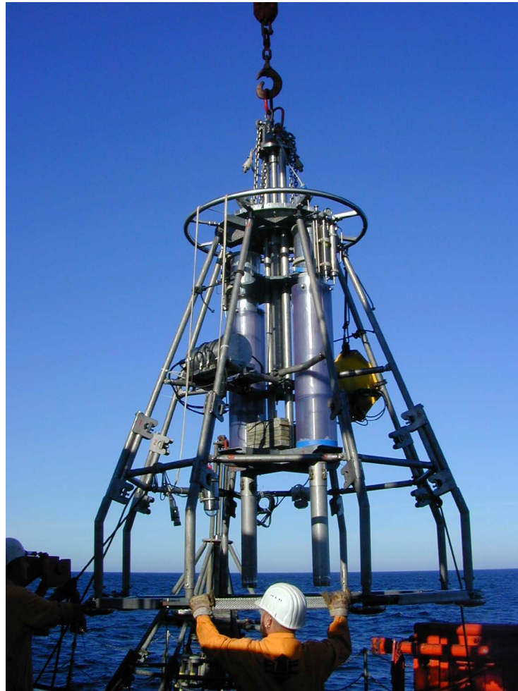
Fig. 5.12.1: Deployment of the MAC with two cores
