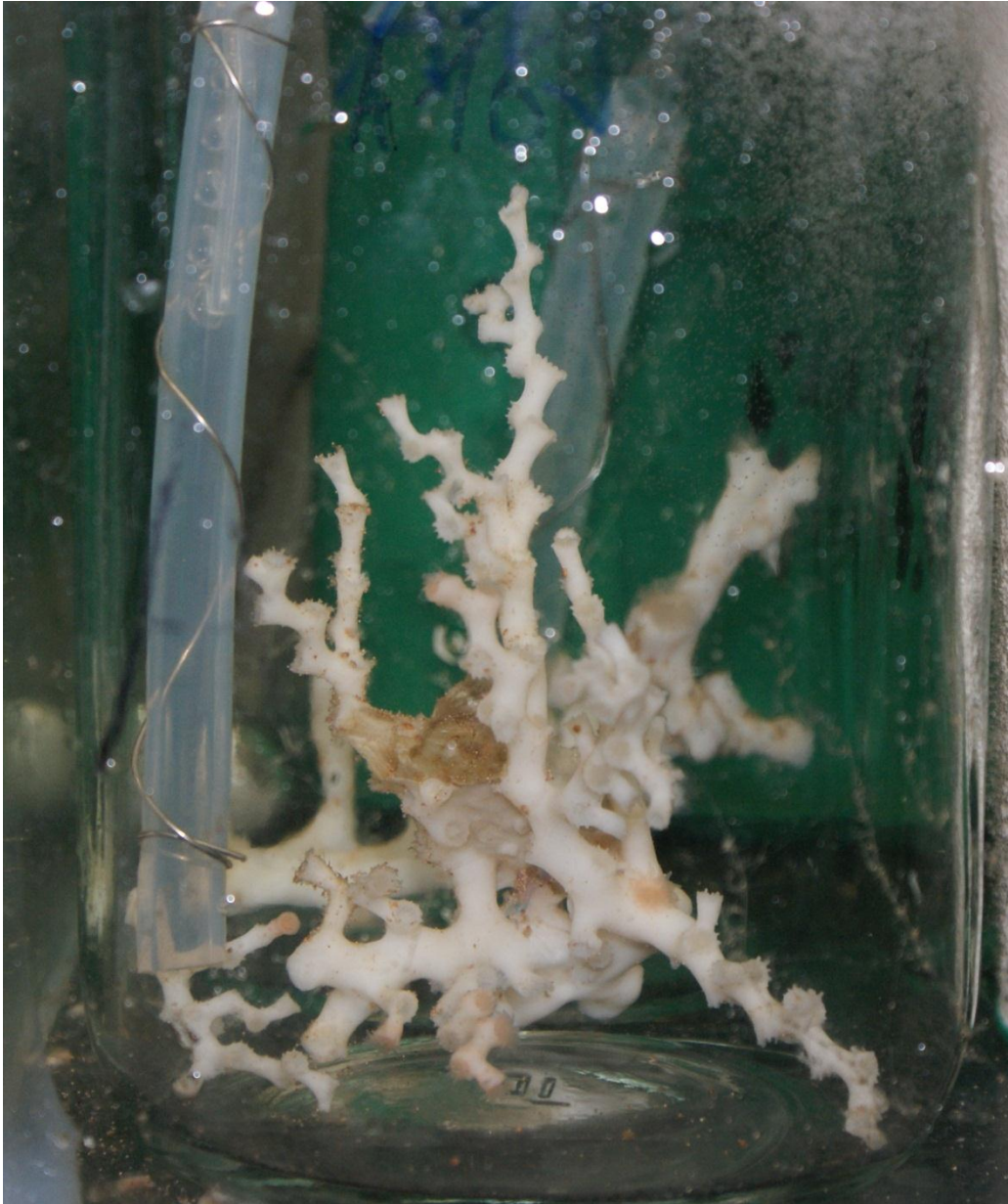
Figure 3: Example of 1L vial containing a Madrepora oculata colony. Observe plastic tube containing thin tube bubbling pCO 2 . Such design aided gas distribution and circulation within vial
