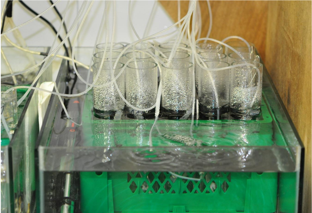
Figure 2: Sample aquaria showing 700ml vials and two thin tubes per vial. One distributing water and the other \text{pCO}_2 gas at relevant concentration. There were four such aquaria (one per \text{pCO}_2 treatment) in this study 2
