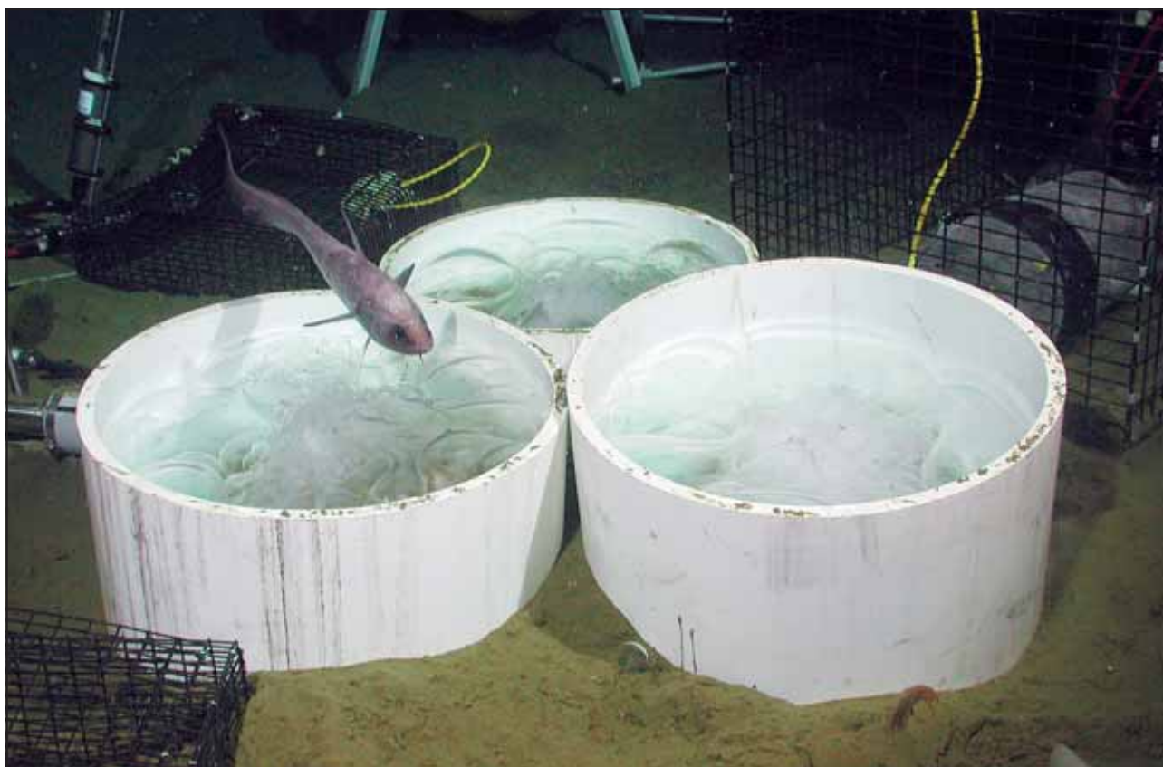
Figure 8.2 Photograph of manipulative deep-sea experiment to evaluate the response of deep-sea organisms to low pH / high p(CO 2 ). Liquid CO 2 (~60 l) was released into PVC tubes (~45 cm diameter) placed on the seafloor at 3600 m depth off central California. The liquid CO 2 dissolved into seawater, producing a high CO 2 , low pH plume that drifted over the seabed and organisms in the sediment or held in cages at different distances from the CO 2 pools (photo credit: J.P. Barry).
