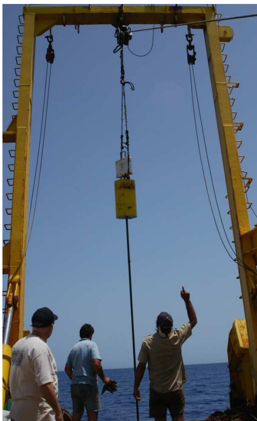
Figure 8.1.1: Recovery of piezometer #310/2 by wireline (left), tip of stinger and hydraulic stab covered by carbonate (right).
