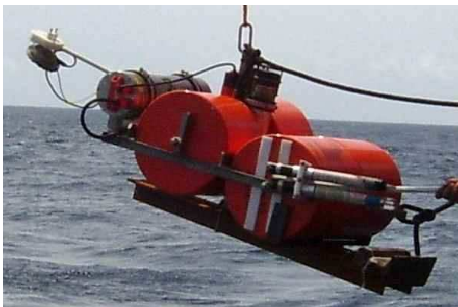
Figure 7.1.1: Ocean-Bottom-Seismometer – OBS - during deployment
