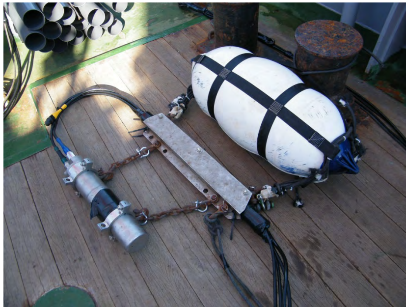
Fig. 13: Micro GI-Gun used during seismic surveying on P395.
