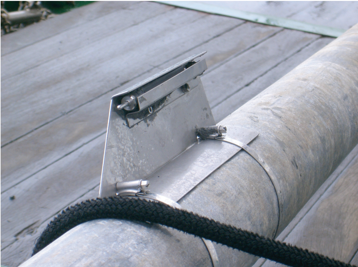
Figure 6.2: Miniaturized temperature loggers (MTLs) were mounted on outriggers attached to the barrel of the gravity corer to determine the thermal regime from which sediment samples were taken. The temperature sensor is located in the tip of the housing.
