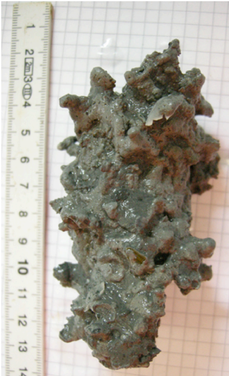
Figure 5.3: Close-up of carbonate chimney found in core P362/2-38-3. The chimney was situated approximately 75 cm below the surface. Bivalve shells are clearly visible and are firmly fixed to the chimney structure.
