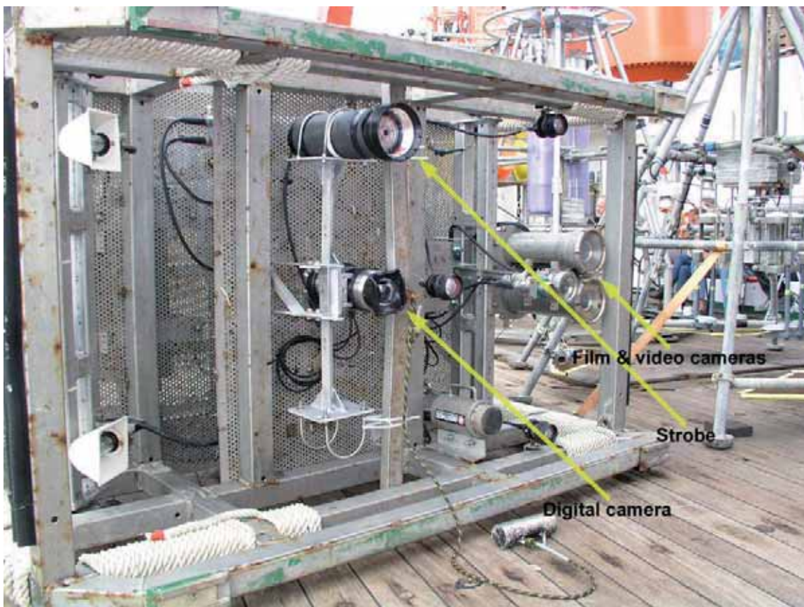
Fig. 32: Ocean Floor Observation System (OFOS) inverted to show camera placements.
