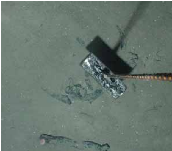
Fig. 33: Bitumen deposits at CK22131. Weight is 20 cm long
