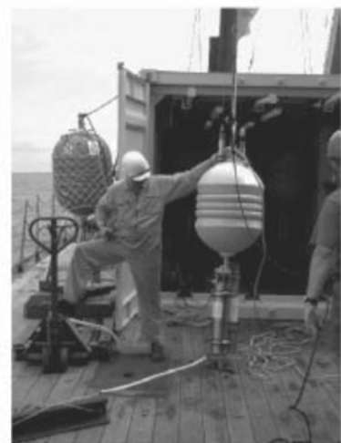
Figure 5.10.2: The GEOMAR OBH ready for deployment.
