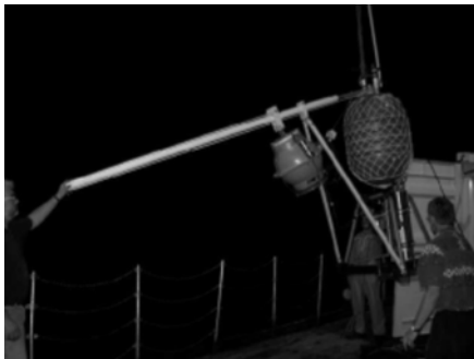
Figure 5.10.6: The GEOMAR broadband seismometer equipped with Webb seismometer at deployment.
