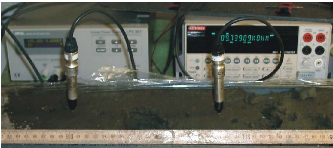
Figure A.HF.2: Two of the five employed needle-probes embedded in the sediments of a split-core, and the linear power supply (left) as well as the digital multimeter (right) in the background.
