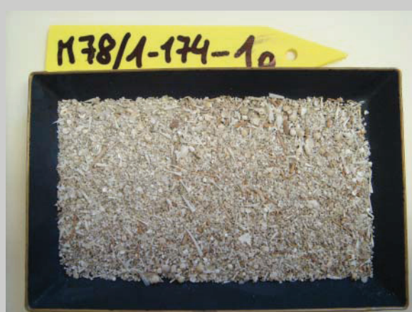
Upper part, grain size fraction &gt; 500 μm
