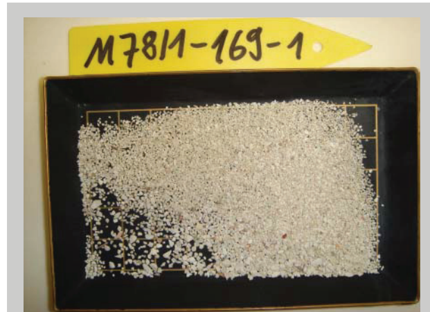
Grain size fraction > 500 µm
