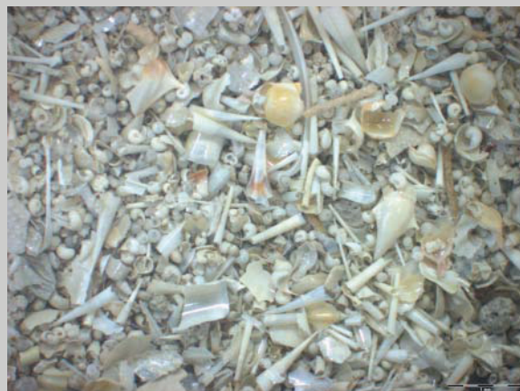
Close-up of grain size fraction &gt; 500 µm
