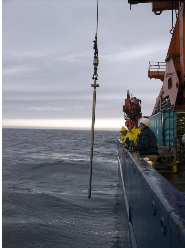
Figure 28: Deployment of the prototype pressure core barrel on RV Meteor
