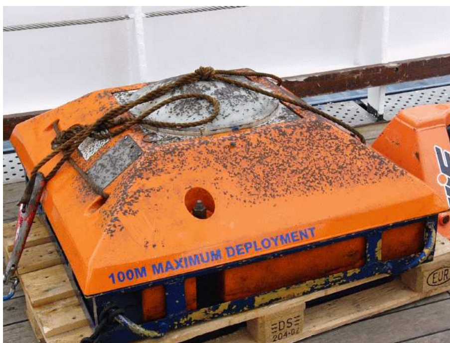
Figure 3.2: Shielded mooring V431 on board ALKOR after its fifth deployment period (09.07.2003 to 15.09.2003).
