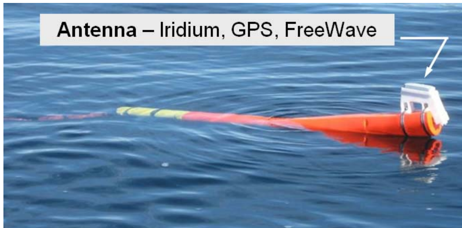
Figure 2: Communication Float in its operating position at the surface. Tank and field studies have shown remarkable stability of this waves ranging from capillary, to wind waves and swell, always keeping the antennas out of the water.
