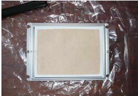
Aerosol filter loaded with Sahara dust sampled 14 -15 Feb 07 near the Cape Verde Islands.
