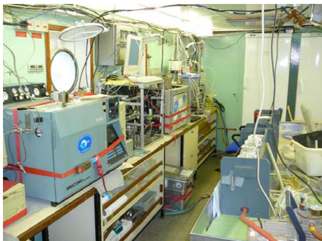
View of Poseidon's wetlab with analytical systems for N 2 O, CH 4 and CO 2 (left) and a filtration device for chlorophyll sampling (right).
