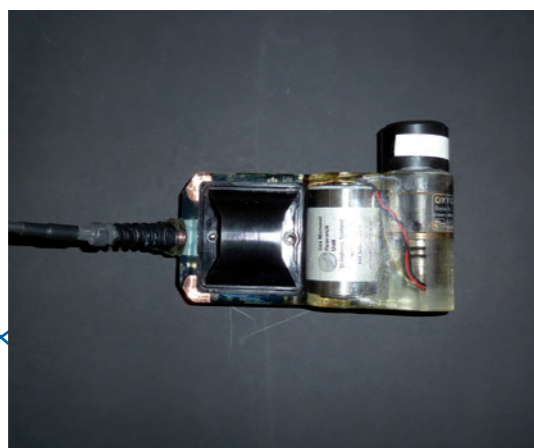
New generation data logger incorporating oxygen sensor.
