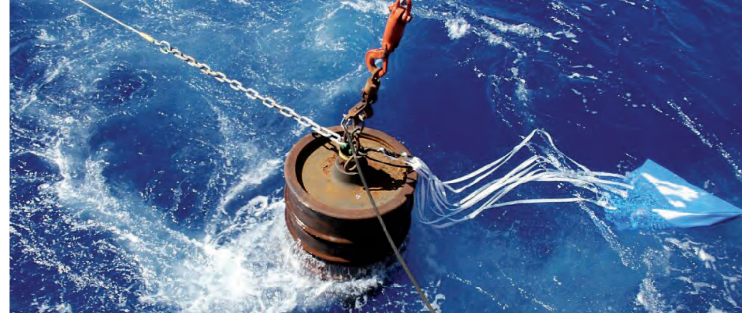
Launch of a mooring anchor dragging along the anchor line. A blue parachute prevents it from sinking too rapidly.
