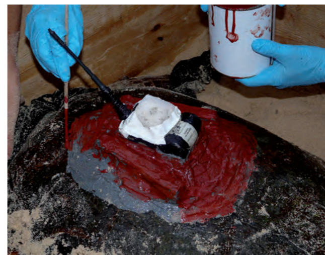
Application of a data recorder on the carapace of the loggerhead sea turtle to register data of its migratory behavior, use of habitat and oceanographic environmental parameters.
