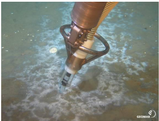
Fig. 4.4.3.1c: Fluid sampling on bacterial mat at fracture zone.
