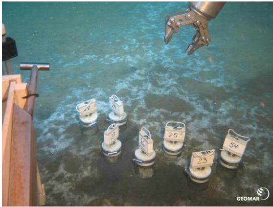
Fig. 4.4.3.1a: Push coring on bacterial mat at fracture zone.
