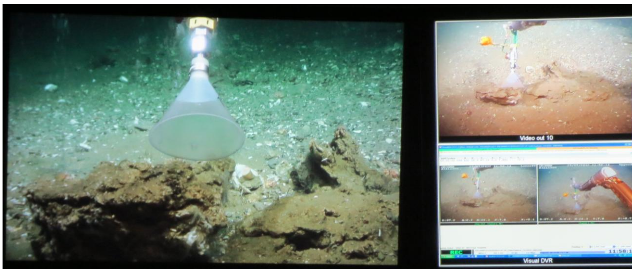
Fig. 4.1.2.2: The gas bubble sampler filled with gas emanated from the seafloor is operated by ROV KIEL 6000.
