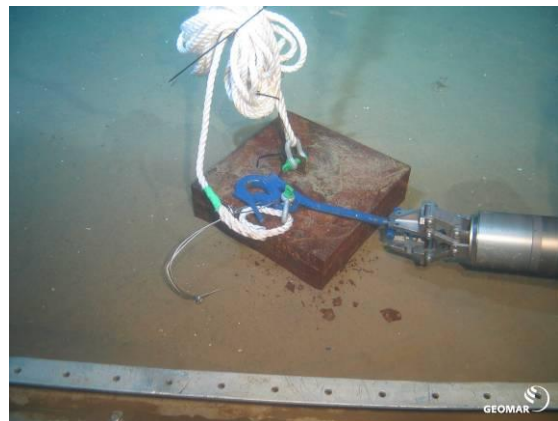
Fig. 4.4.3.1h: Hook-wire-construction for recovering ADCP and anchor weights.
