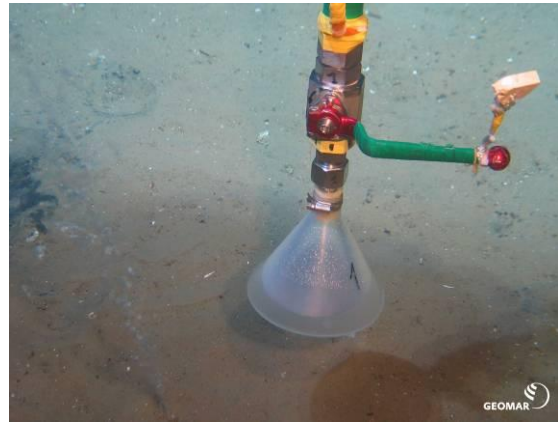
Fig. 4.4.3.1b: Gas sampling at Sleipner.
