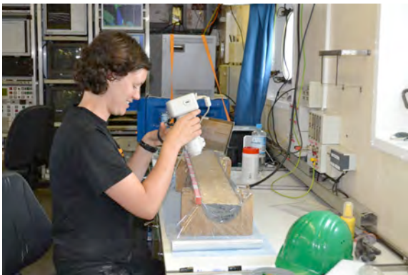
First investigations of a sediment core using a color scanner (photo GEOMAR).
