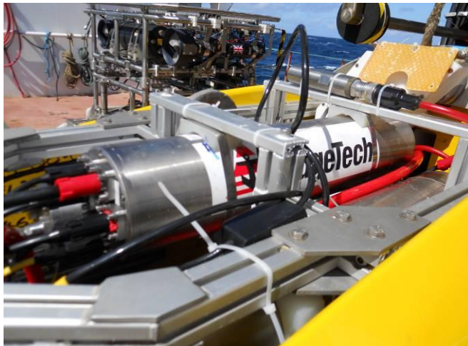
Photo 3. Edgetech electronics mounted in the tail
