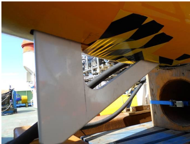
Photo 5. Looking up at the tail section, 'bumble bee' tape covers the aperture cut for the SBP transmitter.
