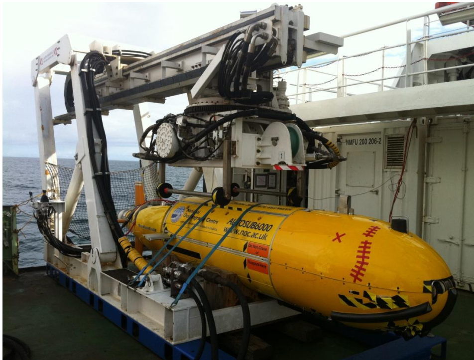
Photo7. The Autosub6000 MKII L&R system installed on the aft deck of the RRS James Cook. The red tape (rather comically) showing the position of some top panel damage due to ship collision on the last recovery
