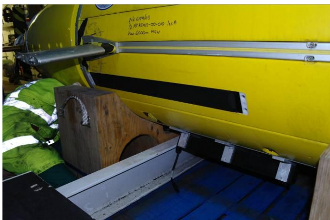
Photo 6. Sub bottom profiler receivers (bottom of photo) mounted outside vehicle
