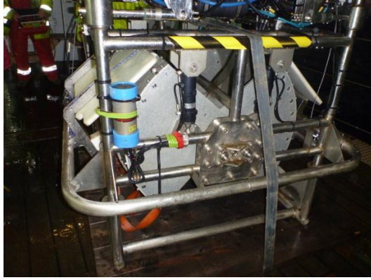
Figure 5.4. EH-sensor (left side) attached to the HyBIS vehicle
