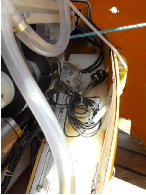
Photo 2 EH sensor on starboard side protruding through panel. PH sensors were also mounted in this position.
