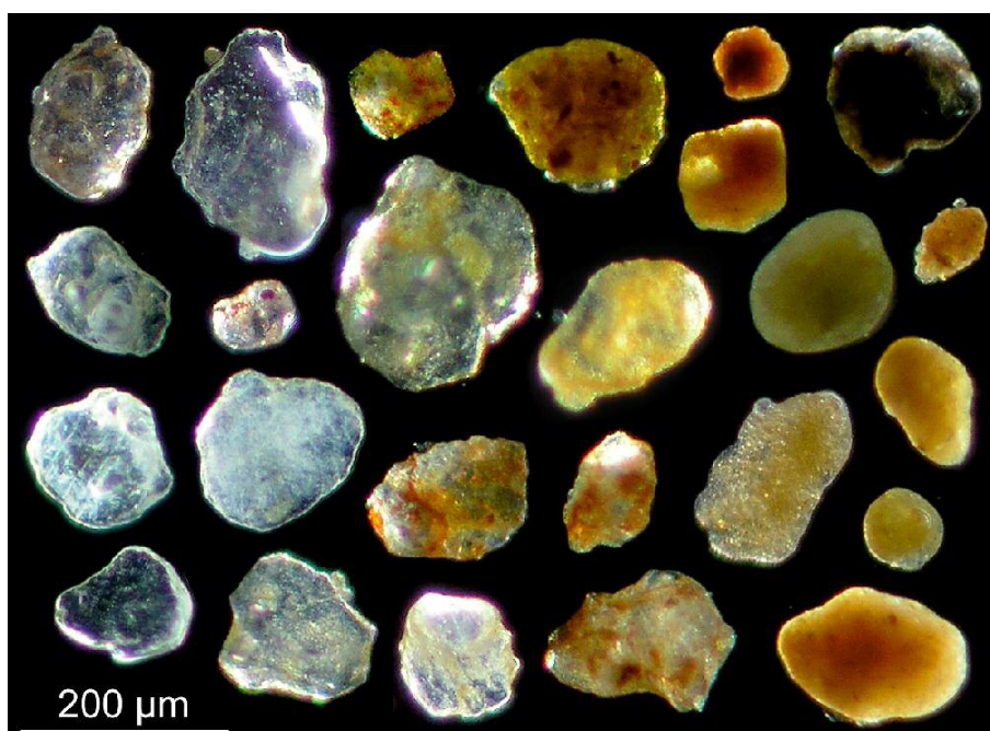
Figure 32: Variety of particle shape and color of airborne Saharan dust. (Kandler et al. (2009))
