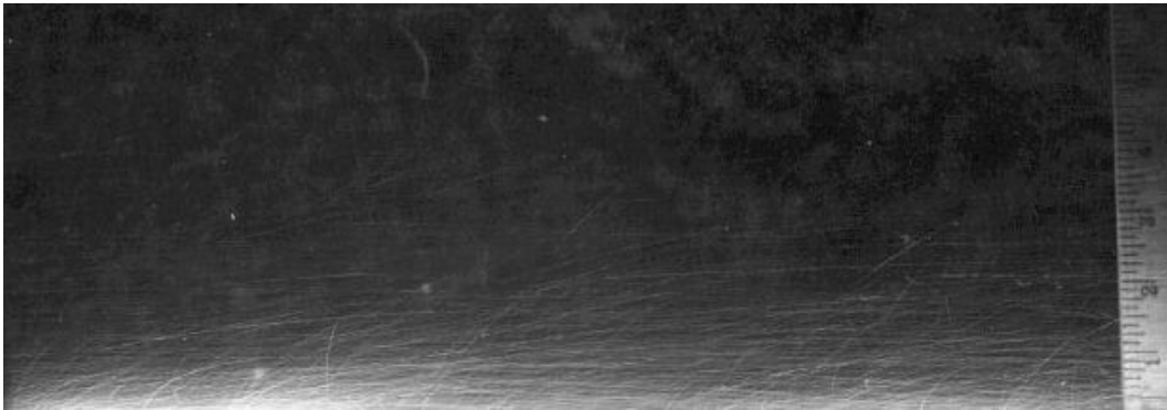
Figure 7: Saltating dune sand in a wind tunnel. (Photo credit: Wind Erosion Research Unit, USDA-ARS, Manhattan, Kansas)
