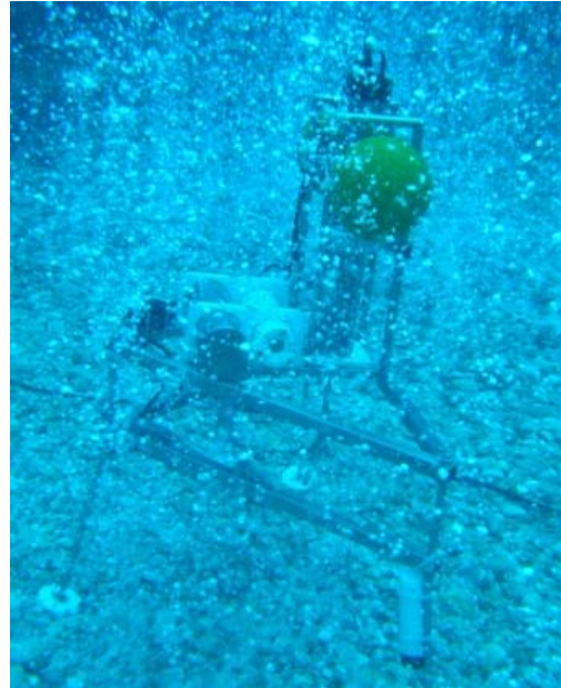
Figure 13: Aquatic Eddy Correlation lander deployed at Bottaro site (© PaCO2 cruise).
