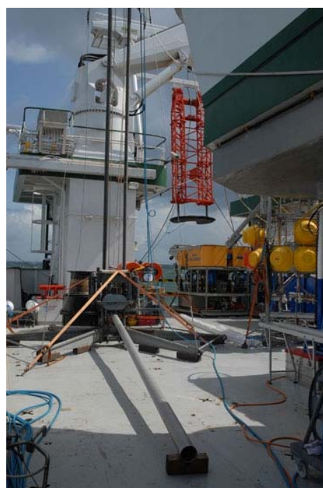
Full working deck on the Celtic Explorer with vibro corer (centre), POZ-Lander und ROV KIEL 6000. Photo: Peter Linke, IFM-GEOMAR
