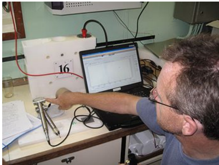
Warner Brückmann calibrating pore pressure sensor for the first piezometer deployment.
