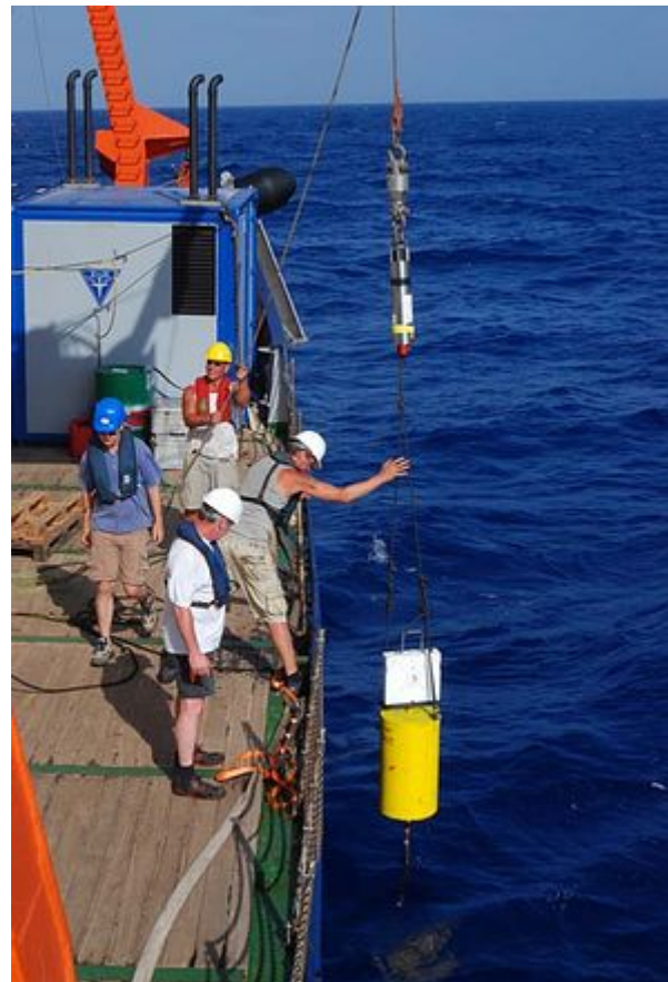
After all components have been assembled, the piezometer is ready for deployment.
