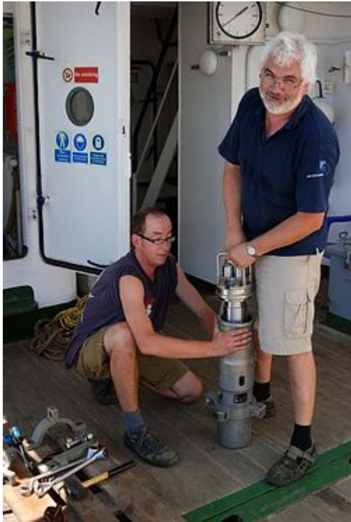
Bernd Herrmann, Ingo Klaucke and Hans-Otto Stange doing maintenance work on the side scan sonar system, which is placed on POSEIDON's afterdeck.
