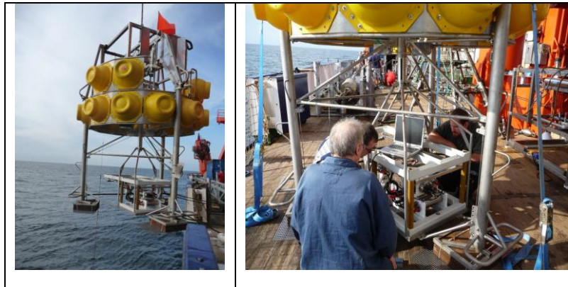
Fig. 2: Left - deployment of a GEOMAR Modular Lander carrying the micro-electrode profiler module; right - the profiler is programmed for deployment.
