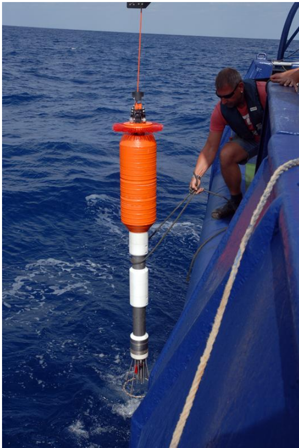
Fig. 11: Deployment of the MSS CTD at the aft of the vessel.
