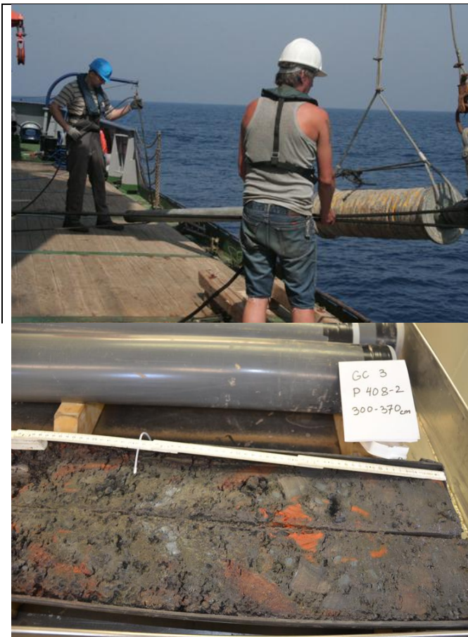
Fig. 5: Deployment of the 6 m long gravity corer (top). Fig. 7: Split cores from the Atlantis II Deep.
