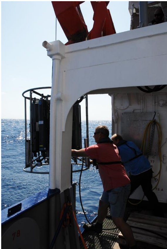
Fig. 8: Deployment of the Video-CTD with various sensors integrated in the water sampler rosette.
