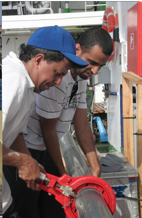
Fig. 6: Cutting of the core liner.
