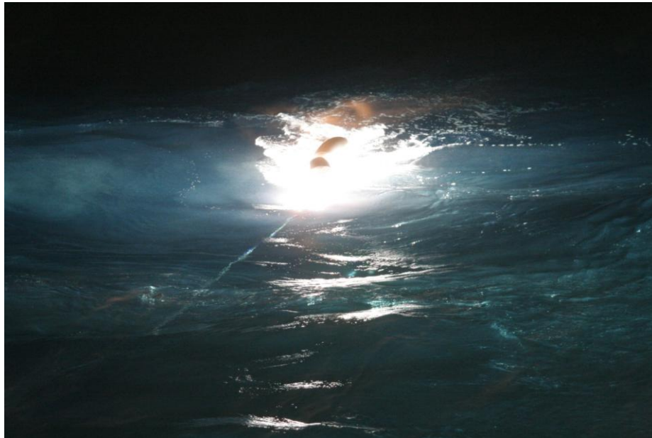
Fig. 2: Delta Sparker (Applied Acoustics) firing at 10 kJ.
