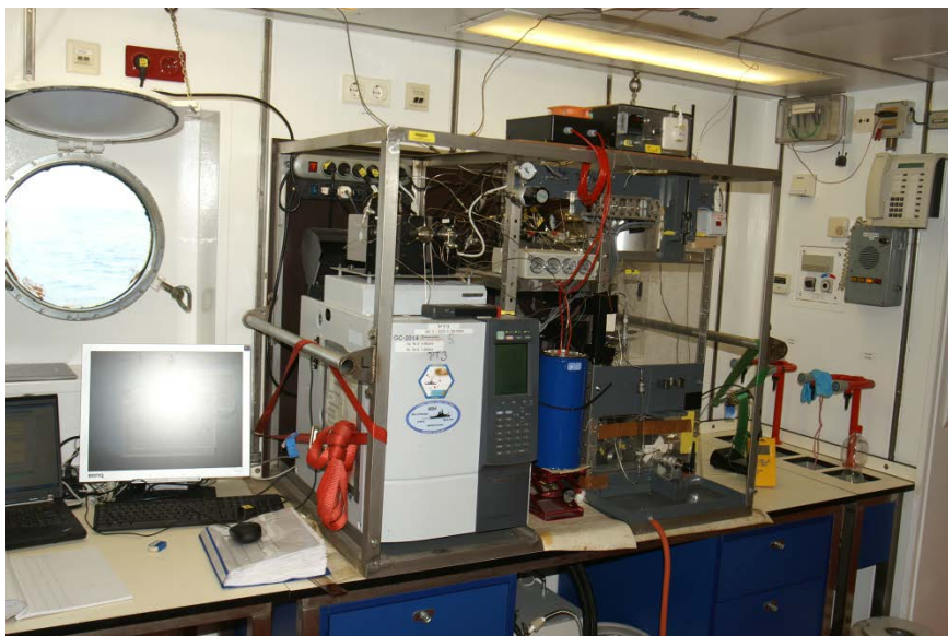
Photo of the instrument used to detect and quantify even minute concentrations of the artificial tracer.
