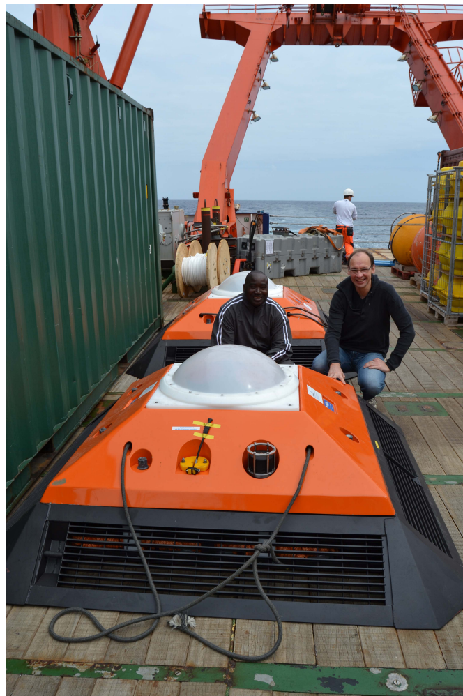
Fig. 1: Two bottom shields equipped with profiling current meters (ADCPs) onboard Meteor prior to the deployment at the shelf off Angola. The instruments were deployed at water depths of 200 m and 500 m and will measure the flow field in the upper ocean until their recovery in 1.5 years.
