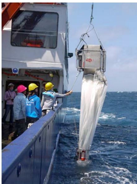
Deployment of a Multi-Net to collect plankton at different water depth.
