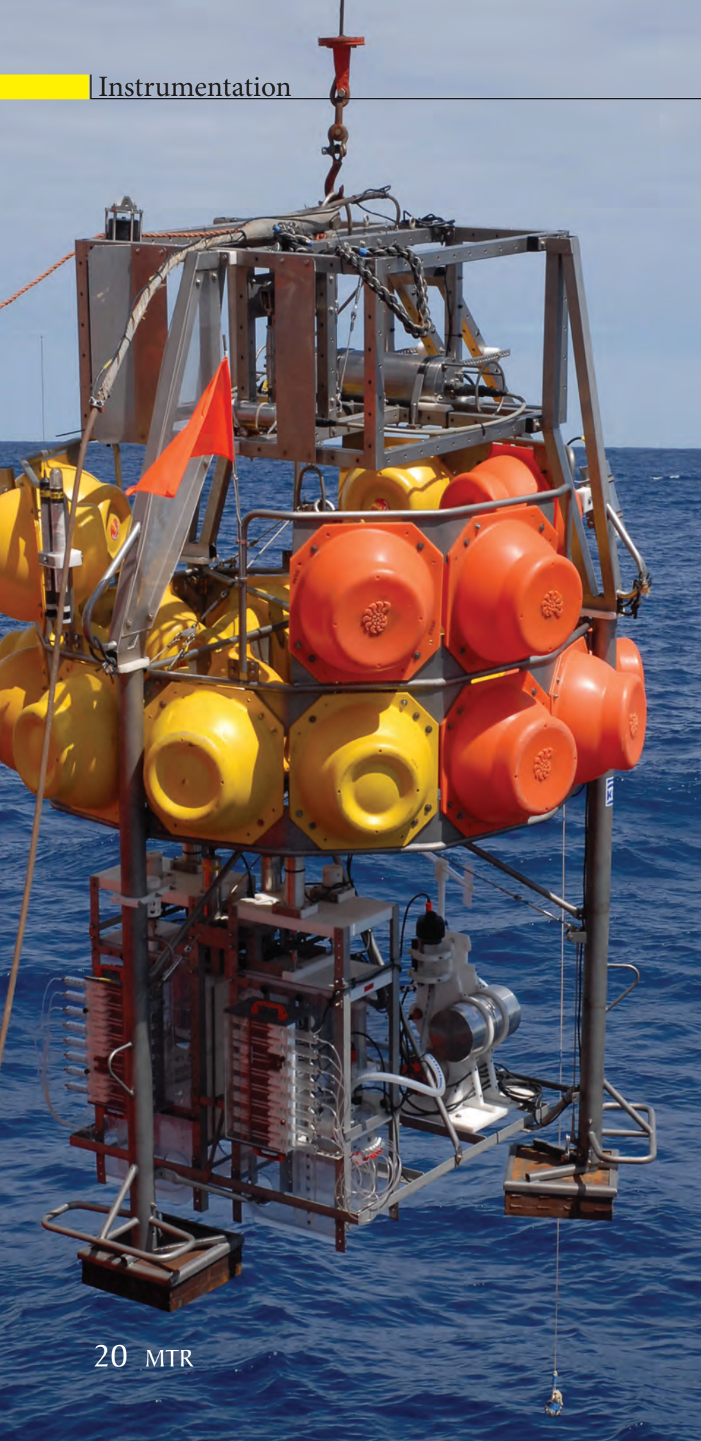
Left: A bottom lander deployment combining an ADCP and the HydroCH4 sensor.
