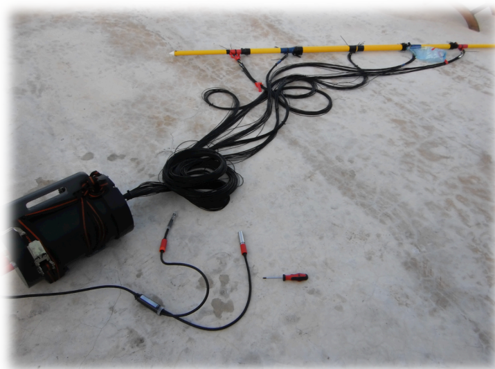
Figure 3: The MuFO system with 100 optodes positioned on a stick in bundles of 20 fibres each.
