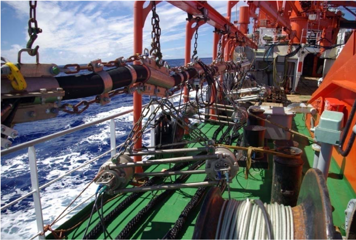
Figure 5.4.2: Picture of the 6 m long port side G-gun Cluster array
