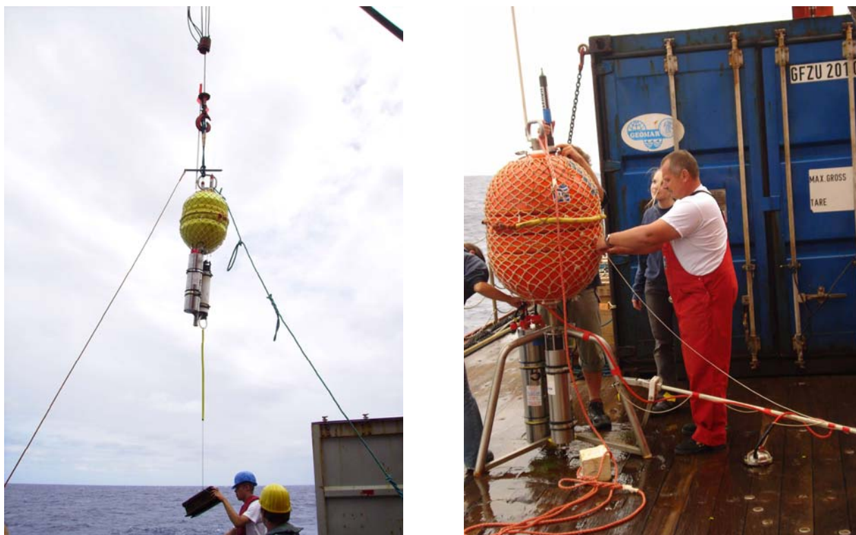
Figure 5.4.1: a) The IFM-GEOMAR OBH ready for deployment, b) the IFM-GEOMAR 3-leg OBS after recovery
