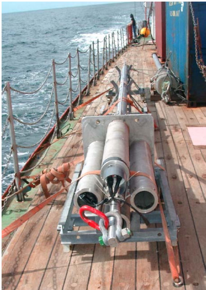
Figure 5.5.2: The 6m-GHF Heat Flow Probe on Deck of R/V Sonne
