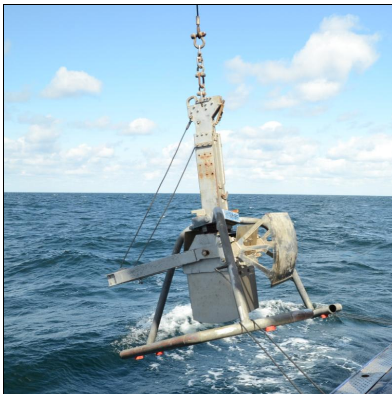
Figure 7: Box corer deploying from the vessel. (Photo: K. Schwarzer)
