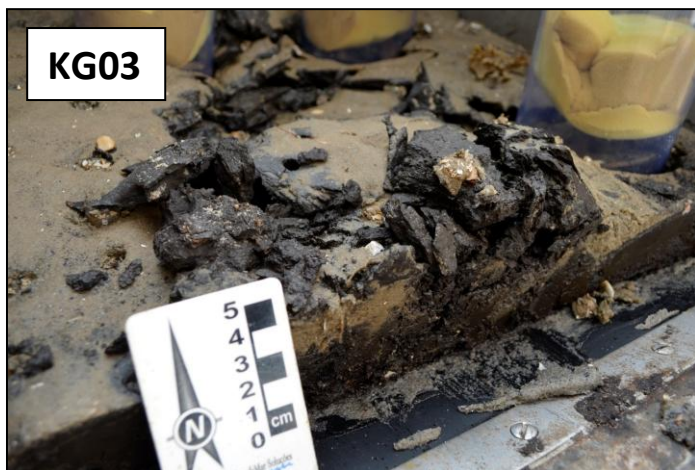
Figure 10: Sediment sample inside a box corer. The sediment is composed of peat, partly covered with medium to fine sand. (Photo: A. Krätschell)
