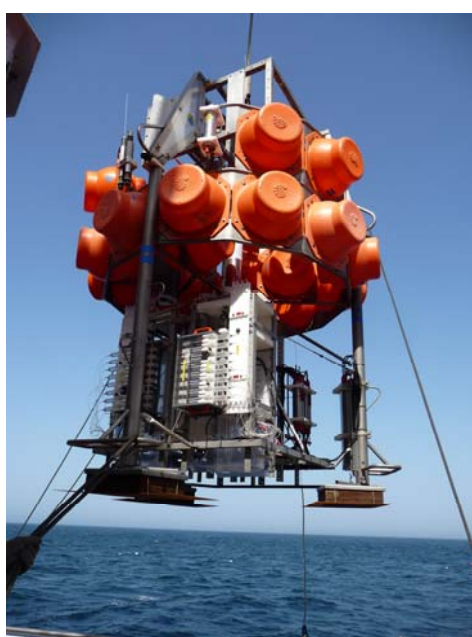
Fig 3: Video-controlled deployment of a BIGO-Lander
