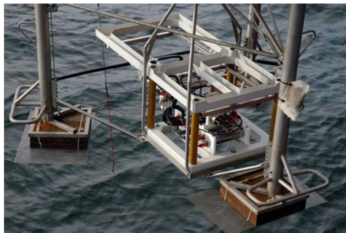
Fig.4: Lander carrying the transecting profiler to conduct 3-dimensional micro-scale measurements of oxygen, sulfide and pH in sediments.
