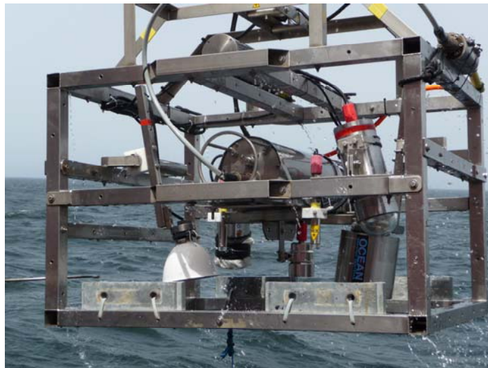
Fig. 1: The OFOS System for seafloor imaging.
