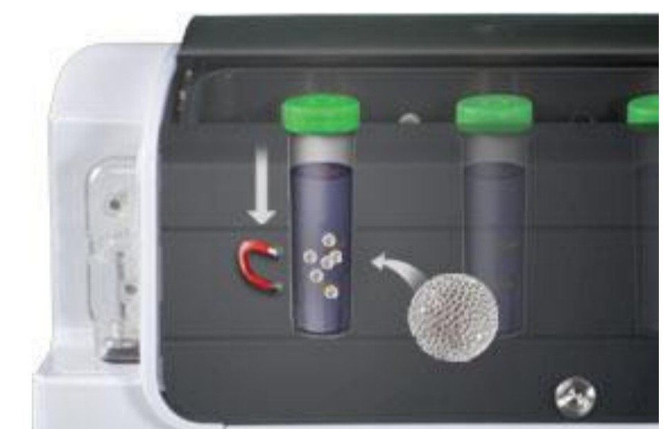
Schematic representation of the incubation chamber with magnetic separator
