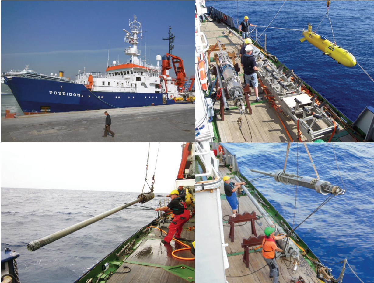
Fig. 4: Research tools used during cruise P462. R/V POSEIDON in the port of Izmir, Turkey (above left); AUV SEAL 5000 m on the working deck during the launching (above right); conventional gravity corer comes back from the seafloor (below left) and the autoclave piston corer (DAPC) deployed from the vessel.
