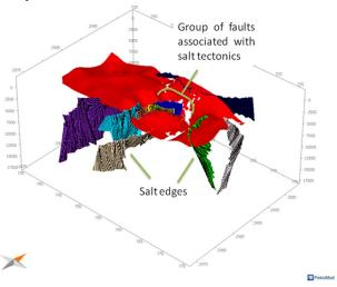
Figure 2: Presence of salt layer (in red) and faultlike structures strongly influences the migration of fluid and gas phases. Migration pathways formed along salt edges (outer part of the model) and faults (central part of the model) provide an efficient high- permeability background for fluid and gas phase transportation.
