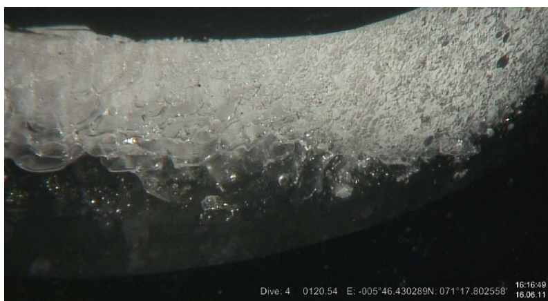
Fig. 9: Dissociation of CO 2 -hydrate sampled at Trollveggen (JMVF) during the ascent of the ROV.
