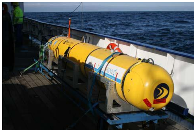
Fig. 29: AUV (AWI) for water column studies above the seafloor.
