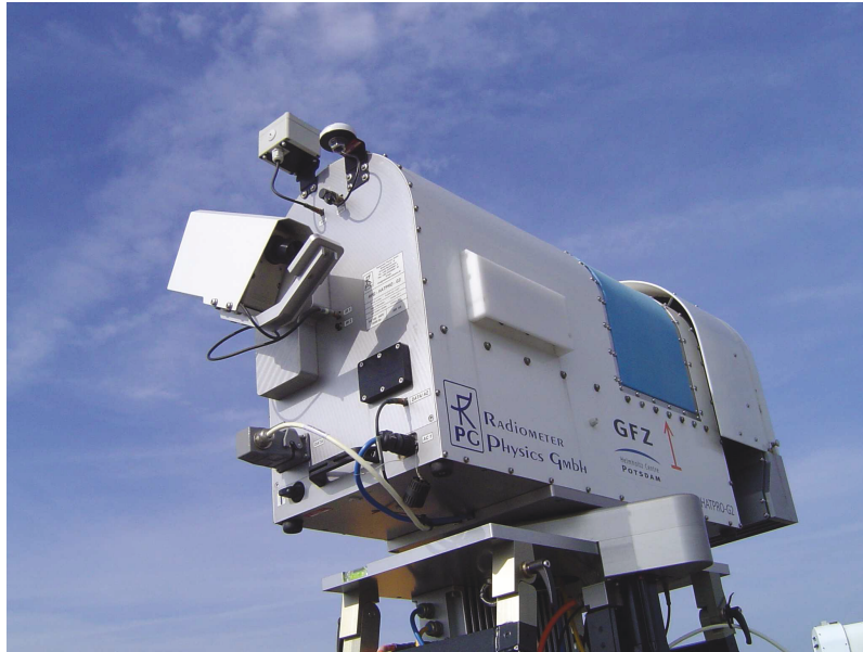
Figure 2.5: Water vapor radiometer (HATPRO) at GFZ.
