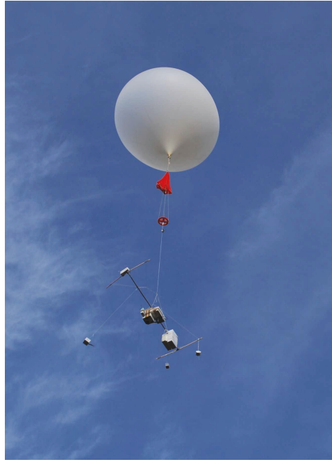
Figure 2.4: Radiosonde from DWD (German Weather Service) carrying different sensors for LUAMI Campaign (2008).
