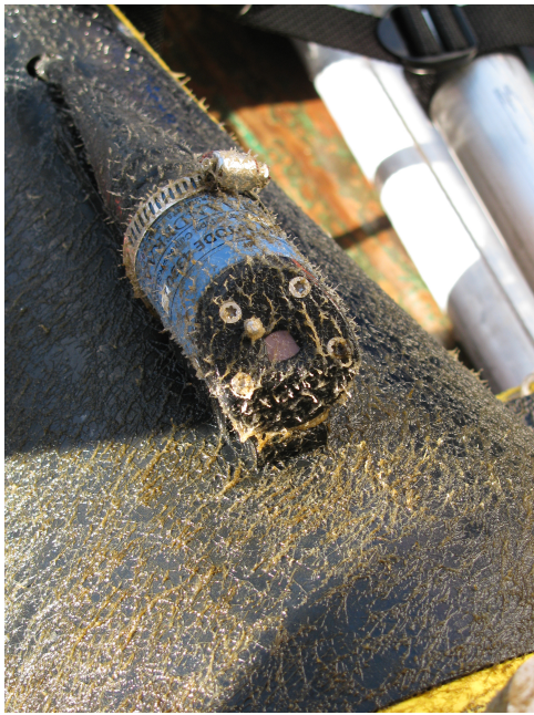
Fig. 3. A thick algal mat covering the Seaglider upon recovery. Growth on the Aanderaa optode may also have contributed to the sensor drift.
